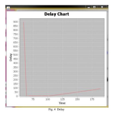
Figure 4 shows delay over simulation time (miliseconds). Initial delay is greater due to the time required to encrypt data and digitally sign it. After system starts sending packets delay is reduced exponentially
